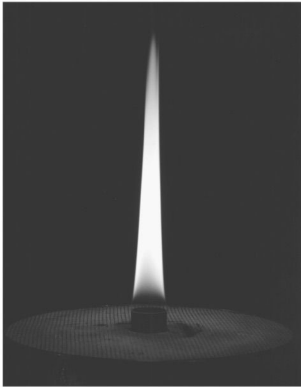
Figure 9.6 Laminar ethylene jet diffusion flame. Note soot "wings" at sides of the flame near the tip. | SOURCE: Photograph courtesy of R. J. Santoro.
