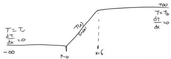
$$-\dot{m}''_c \Delta h_c = cp \dot{m}'' \frac{dT}{dx} - \frac{d}{dx} \left( \rho D_{cp} \frac{dT}{dx} \right)$$
